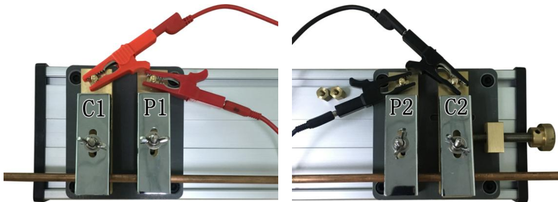
▲Schematic diagram of connection between TX-300B and TXJ-150 micro fixture
